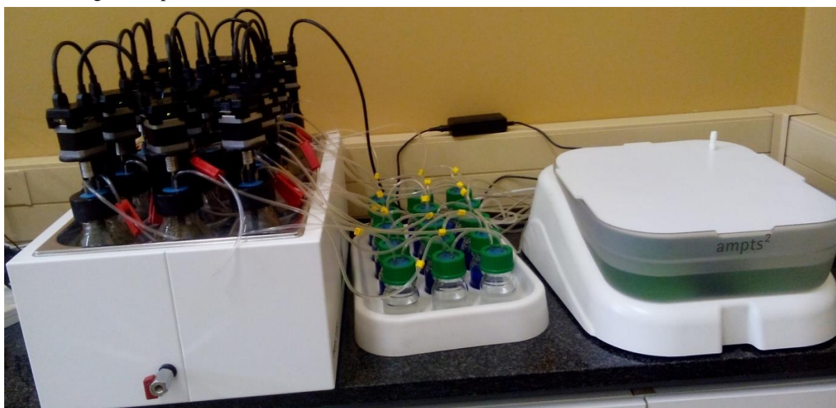
Fig. 1: BMP Assay setup (Bioprocess Control AMPTS II) in the lab- (i) digester, (ii) CO 2 fixing unit, and (iii) gas collecting unit
