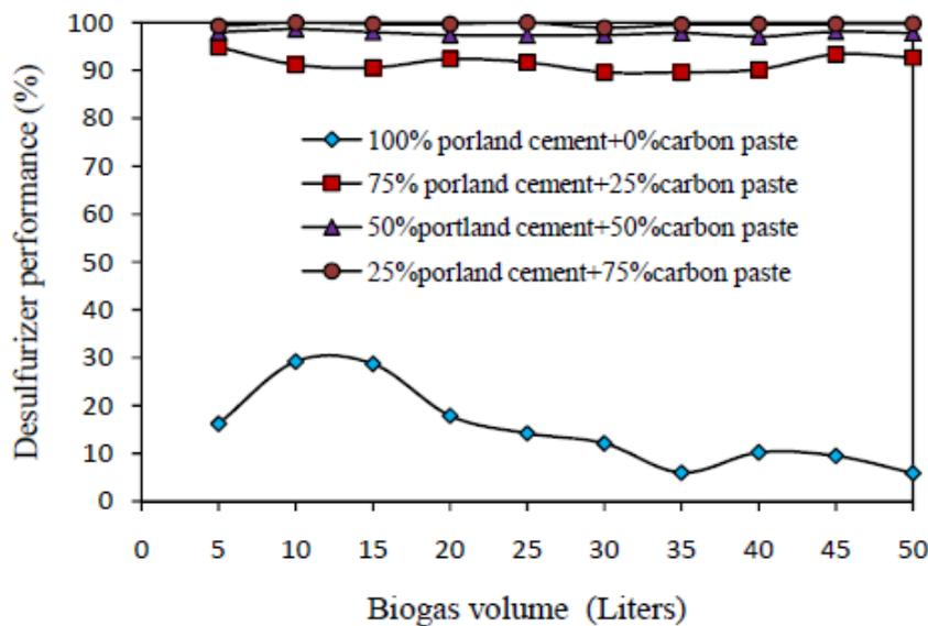
Fig. 4: Effect of mass fraction of carbon paste in Portland cement (PC) on performance of biogas desulfurizer
