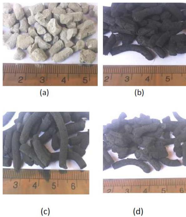
Fig. 2: Dry mixture pellets of carbon paste from used zinc-carbon battery mixed with Portland cement (PC). (a). 0% carbon + 100% PC, (b) 25% carbon + 75% PC, (c) 50% carbon + 50% PC, and (d) 75% carbon + 25% PC.
