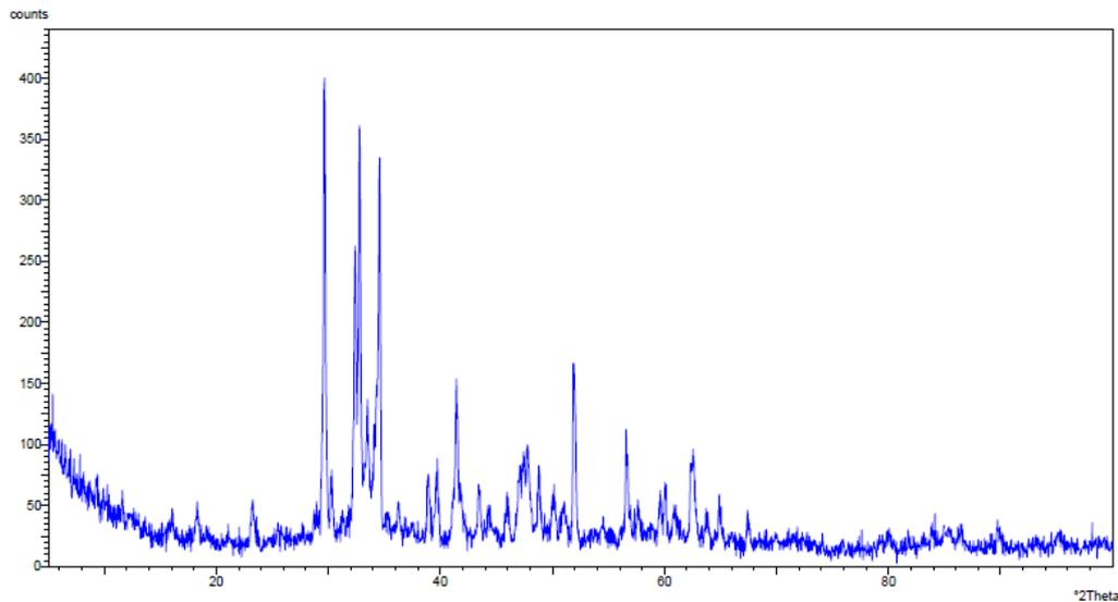
Fig. 5: Result of X ray diffractometer (XRD) on Portland cement. The composition mainly (65%) is calcite ( $\text{CaCO}_3$ )
