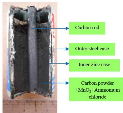
Fig. 1: Inner side of zinc-carbon battery
