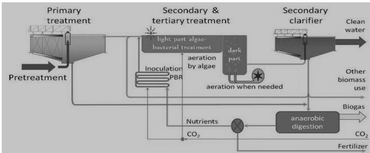
Fig. 3: Example of Flow chart incorporating algae based treatment as part of secondary treatment in a conventional wastewater treatment plant
