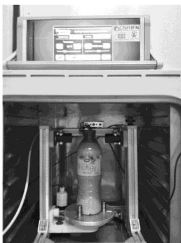
Fig. 1: The laboratory device constructed for non-destructive measurement of CO<sub>2</sub> content in packages of fermented milk products.
