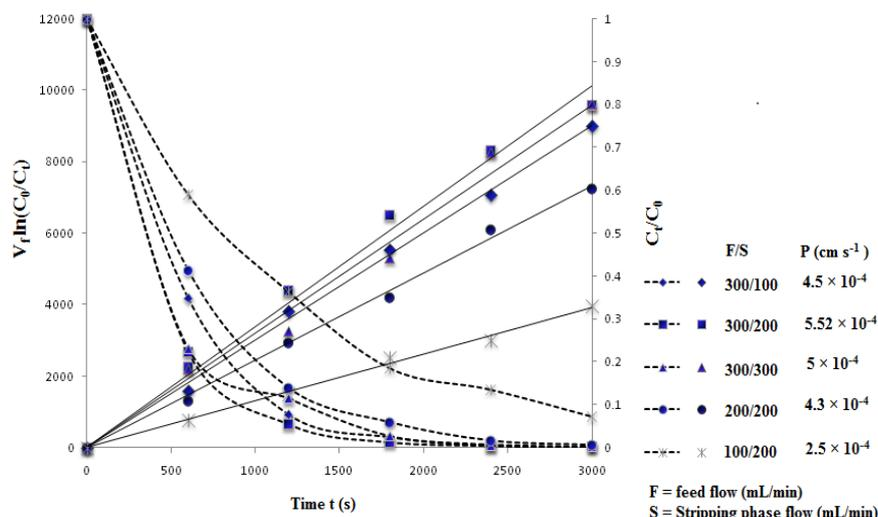
Fig. 2: Effect of feed and pseudo emulsion phase flow rates on the extraction of p-nitrophenol through PEHFSD.
