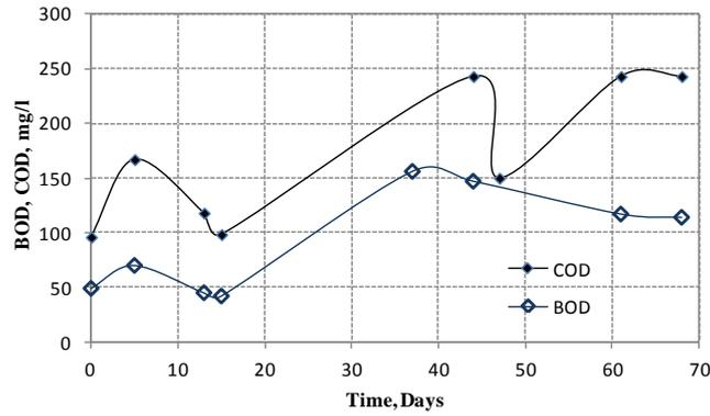
Fig. 4: BOD and COD effluent concentrations during column experiments.
