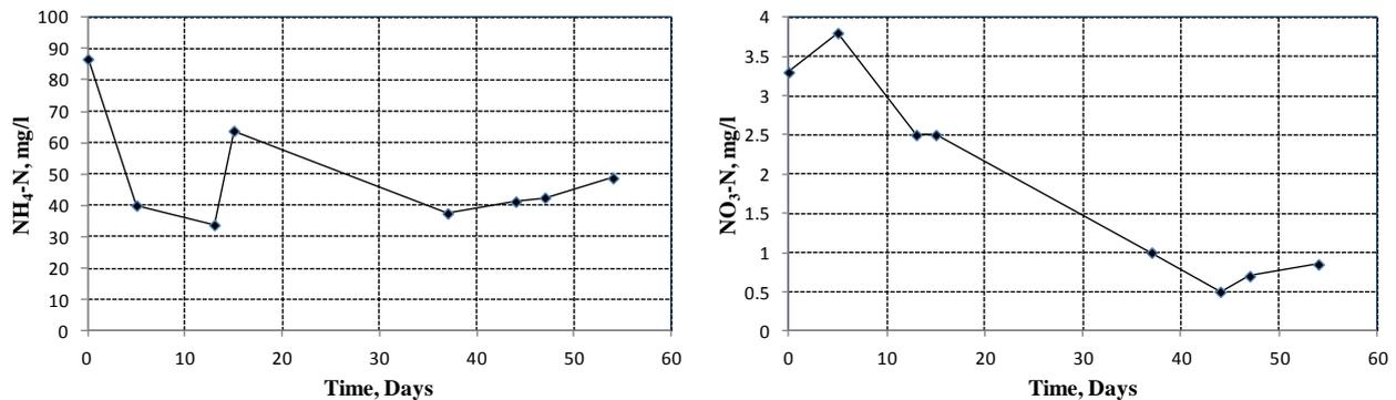
Fig. 6: Ammonia nitrogen and nitrate nitrogen effluent concentration during column experiments.
