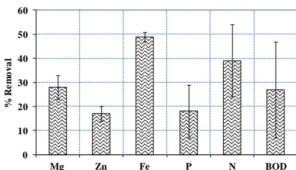
Fig. 2: Peat column removal efficiency for magnesium (Mg), zinc (Zn), iron (Fe), phosphorous (P as  $\text{PO}_4$ ), nitrogen (N as  $\text{NO}_3$ ), and 5-day biochemical oxygen demand (BOD).
