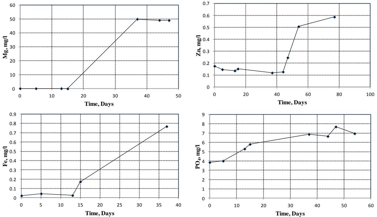
Fig. 5: Column breakthrough curves for Mg, Fe, Zn, and PO<sub>4</sub>.
