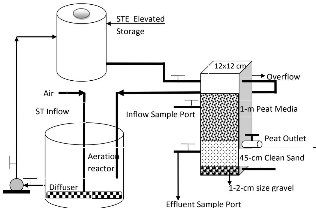
Fig. 1: Schematic diagram of peat adsorption and absorption system.
