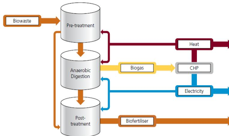
Fig. 1: Overview of an Anaerobic Digestion System [5]
