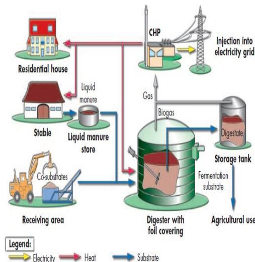
Fig. 2: Conversion of biogas to heat and power [16]
