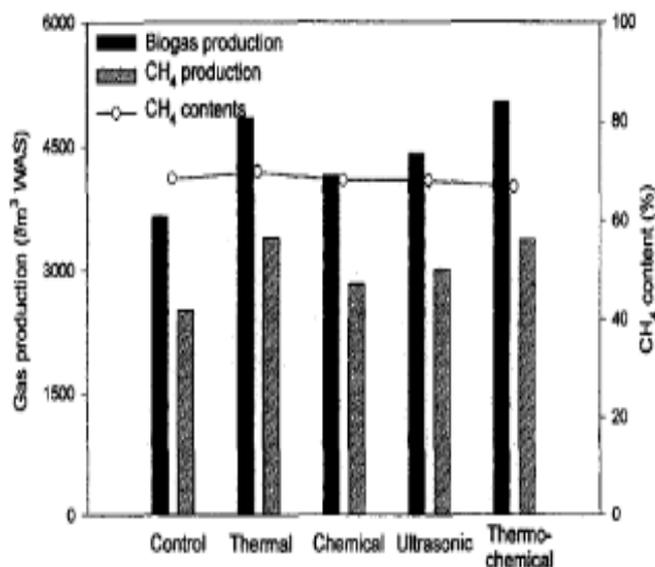
Fig. 3: How pretreatment methods improves biogas production [21]
