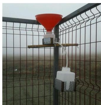
Fig. 1.b: Precipitation collection device
