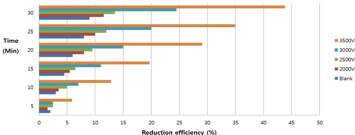
Fig. 1: Hydrogen Sulfide Reduction efficiency to Different Voltages
