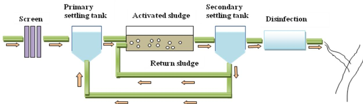
Fig. 1: General description of domestic wastewater treatment plant
