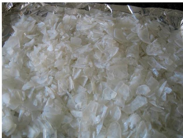
Fig. 1: Titanium dioxide coated broken glass units
