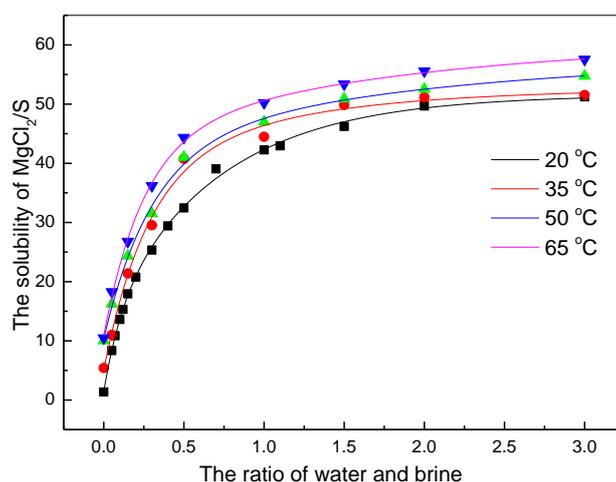
Fig. 9: The solubility of magnesium chloride hexahydrate of under different dilution ratios of old bitterm
