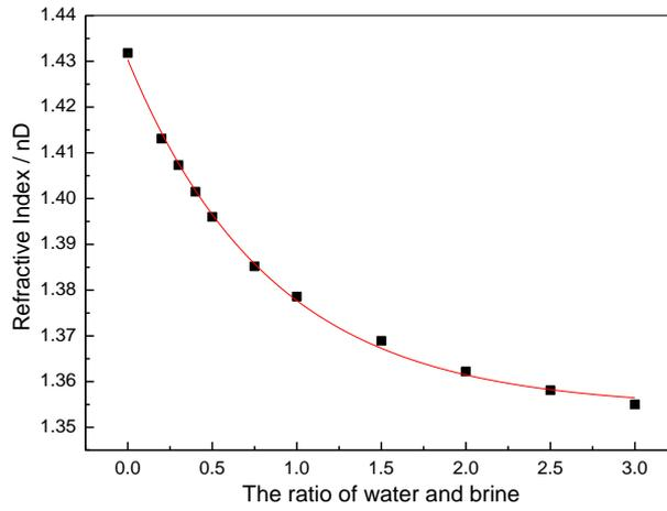
Fig. 6: The refractive index of the brine of different dilution ratio
