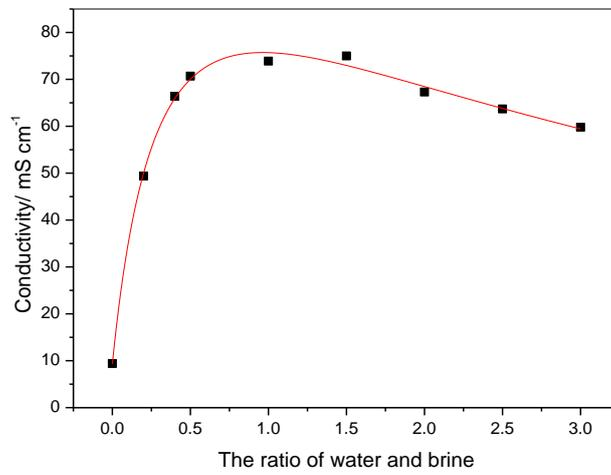
Fig. 7: The conductivity of the brine of different dilution ratio
