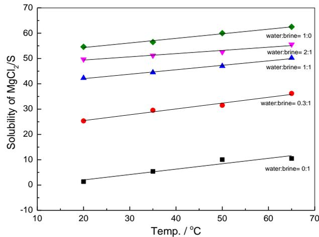
Fig. 8: The solubility of magnesium chloride hexahydrate under the different temperature
