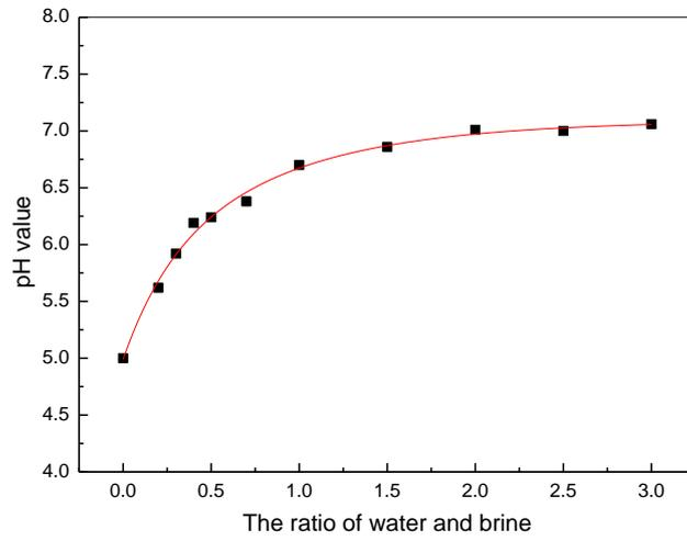
Fig. 4: pH value of the brine of different dilution ratio
