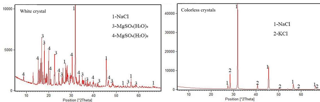
Fig. 2: XRD image of different crystalline low-grade solid potassium deposit
