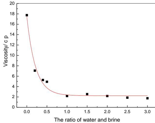
Fig. 5: The viscosity of the brine of different dilution ratio
