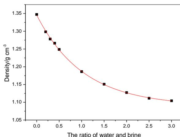
Fig. 1: The density of the brine of different dilution ratio
