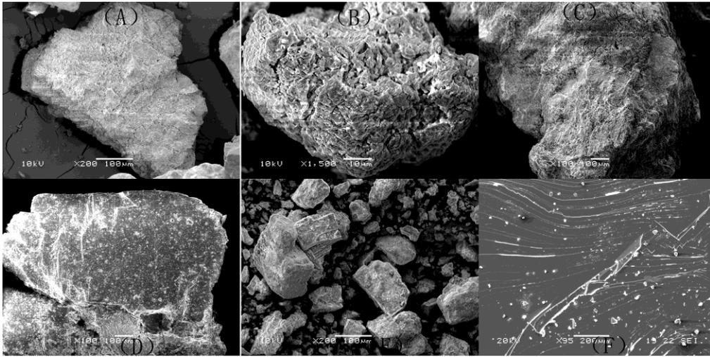
Fig. 3: SEM image of low-grade solid potassium of magnesium sulfate subtypes
