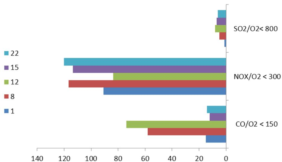
Fig. 1: Results obtained from measurement of gases emitting from chimneys
