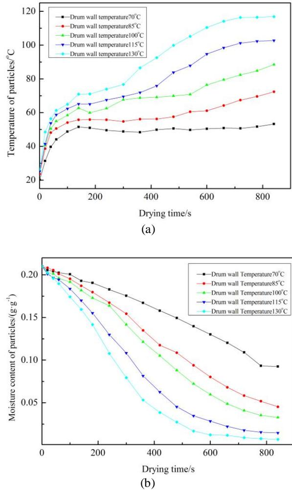
Fig. 3: Moisture content and temperature of cut stem particles under different temperature of drum wall.
