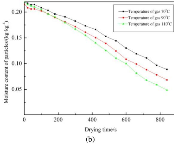
Fig. 5: Moisture content and temperature of cut stem particles under different temperature of gas flow.
