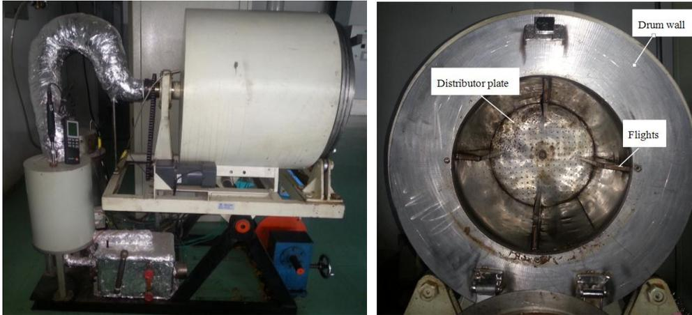
Fig. 2: Structure of the experimental set up
