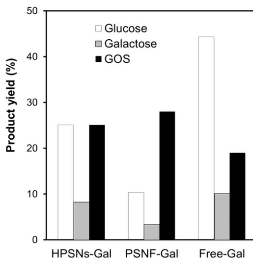
Fig. 4: The profile of product distributions by HPSNs-Gal, PSNF-Gal and free-Gal at 400 g/l initial lactose concentration. (Enzyme concentration: 2 mg/ml in pH 7 phosphate buffer solution, incubated at 37 °C).
