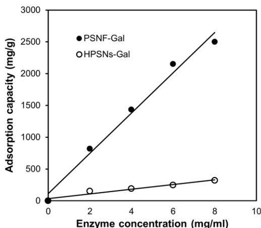
Fig. 2: The comparison of adsorption capacity between HPSNs-Gal and PSNF-Gal at different enzyme concentrations.
