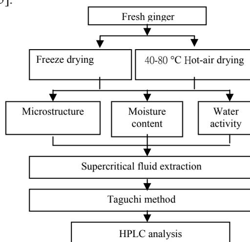
Fig. 1. Schematic representation of extraction and isolation of 6-shogaol compound from dried ginger slices by Supercritical fluid extraction.
