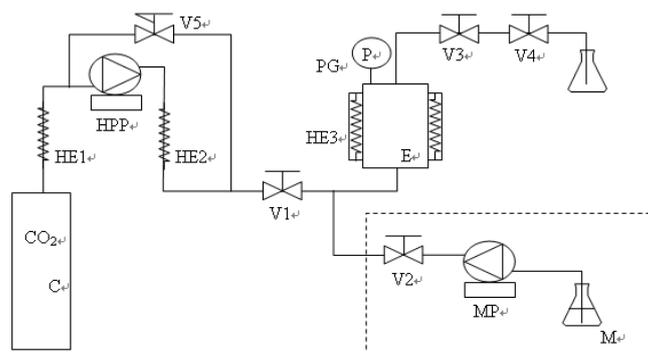
Fig. 2. Scheme of supercritical carbon dioxide extraction equipment at batch-stirred apparatus for synthesis under high pressure: (C) CO<sub>2</sub> tank, (E) Extract vessel, (HE1-3) Heat exchangers, (HPP) High pressure pump, (M) Modifier, (MP) Modifier pump, (PG) Pressure gauges, (V1-3) exhaust valve, (V4) Needle valve, (V5) Back pressure valve.
