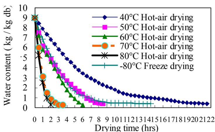
Fig. 3. The drying characteristic curve of ginger slices under different drying temperature.
