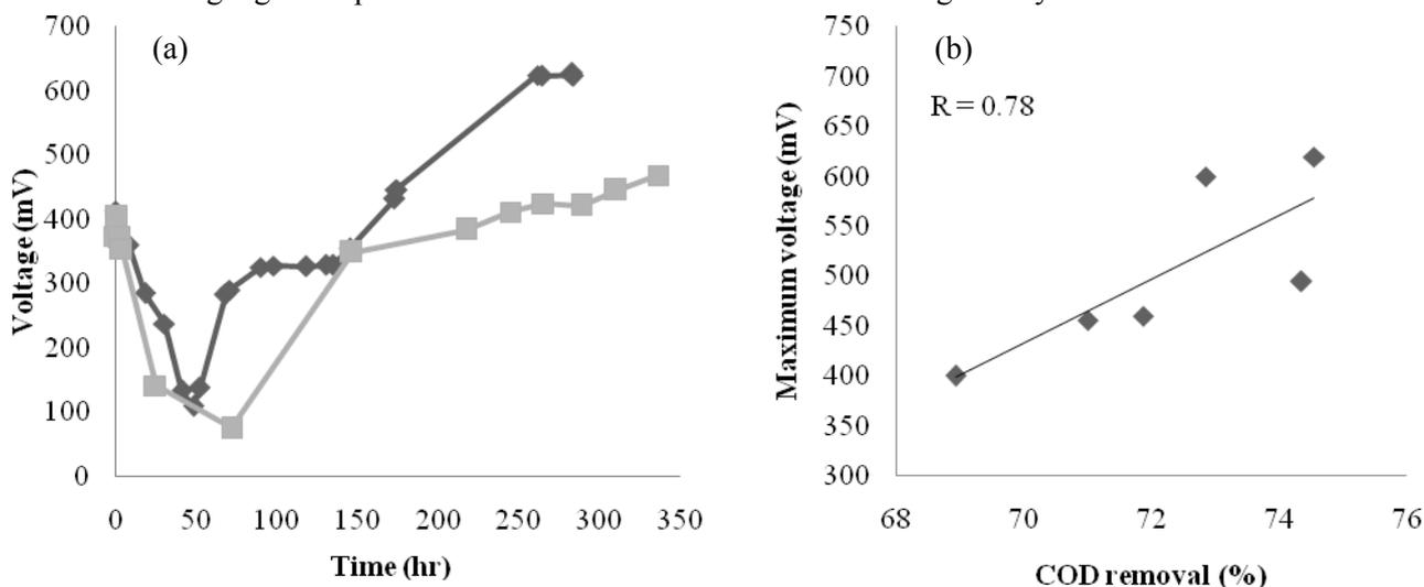
Fig. 3 : (a) Cell voltage of MFC when adding glucose as a co-substrate (◆) compared with the control (■) and (b) correlation between maximum MFC cell voltage and percentage of COD removal of the wastewater.
