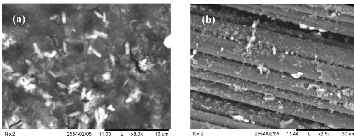
Fig. 2 : Scanning electron microscope (SEM) images of (a) graphite and (b) carbon cloth electrodes in anode chamber after electrogenic digestion for 12 days.
