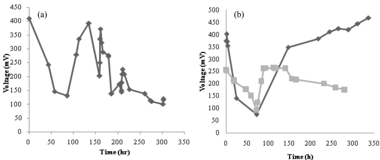
Fig. 1 : (A) Effect of nitrogen purging in anode chamber on the cell voltage at 160 hr, 180 hr and 210 hr, and (B) cell voltage of MFC when graphite (◆) and carbon cloth (■) were used as electrodes.
