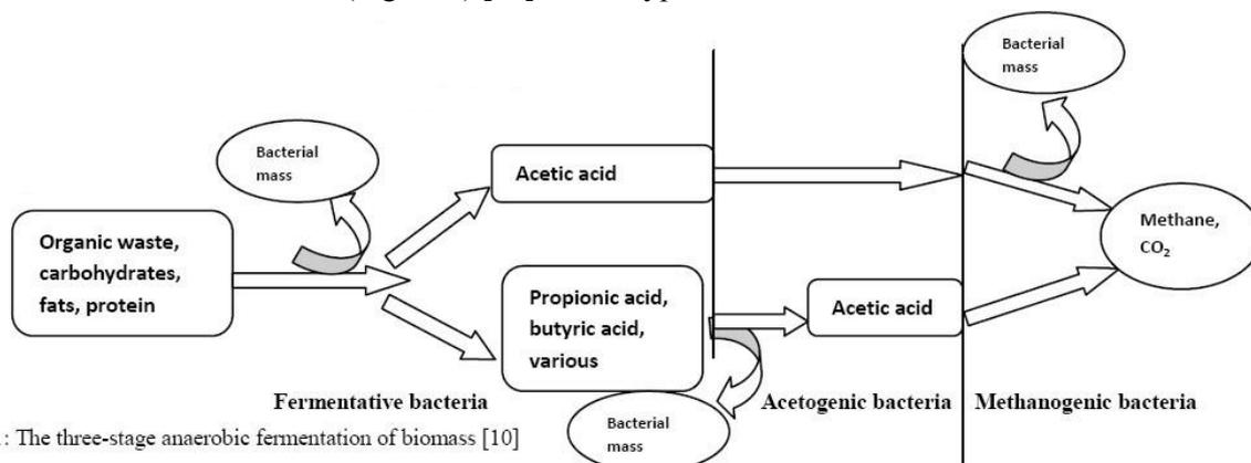
Figure 1: The three-stage anaerobic fermentation of biomass [10]
