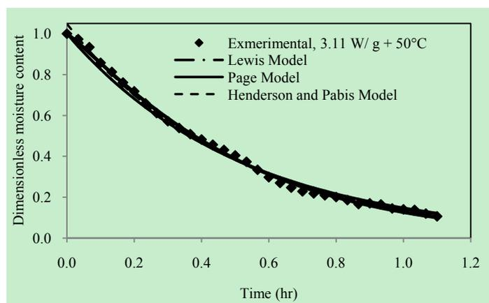
Fig. 6. Comparison of experimental and calculated dimensionless moisture content of tomato slices as a function of drying time ( $T = 50^{\circ}\text{C}$  and microwave power density of 3.11 W g-1)
