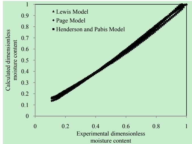
Fig. 9. Comparison of experimental and calculated dimensionless moisture content of tomato slices (T = 40°C)
