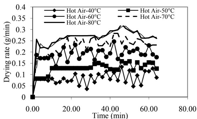
Fig. 4. Drying rate of tomato slices changes with drying time
