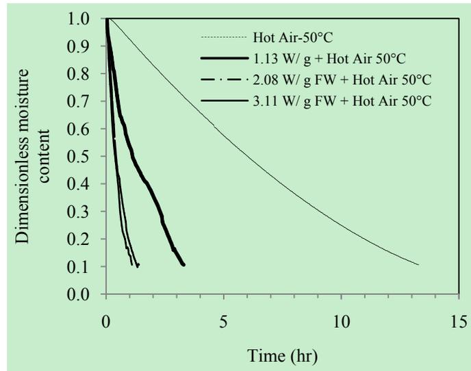
Fig. 1. Moisture content of tomato slices changes with microwave power density and time
