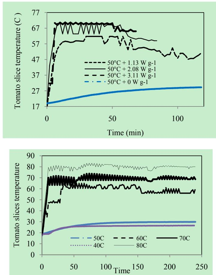
Fig. 5a,b. Tomato slice temperature during drying with air velocity at 1.0 m/s, air temperature at 40, 50, 60, 70 and 80°C, and power density at 1.13, 2.08 and 3.11 W g<sup>-1</sup>.
