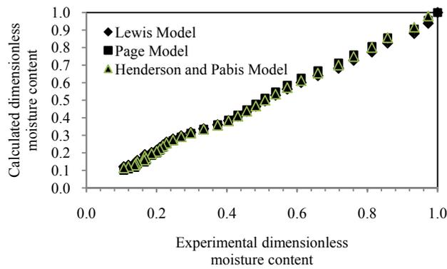
Fig. 7. Comparison of experimental and calculated dimensionless moisture content of tomato slices ( $T = 50^{\circ}\text{C}$  and microwave power density of  $3.11 \text{ W g}^{-1}$ ).
