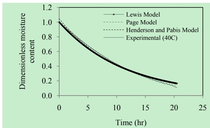
Fig. 8. Comparison of experimental and calculated dimensionless moisture content of tomato slices (T = 40°C)
