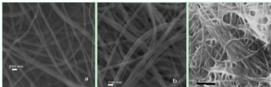
Figure 1: Scanning Electron Micrograph of PAN nanofibrous membrane (a) original nanofibrous membrane (7.5 wt. %) PAN (b) 10% GA treated PANNFM (c) chitosanase immobilized on GA treated NFM
