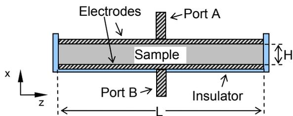
Fig. 3: Cross-sectional view of the static treatment chamber equipped with vertical-aligned conductive plates with  $H$  and  $L$  of 0.5 cm and 10 cm, respectively. Pulses are delivered into port A.
