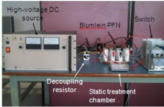
Fig. 1: Experiment setup of the high-intensity nsPEF system.
