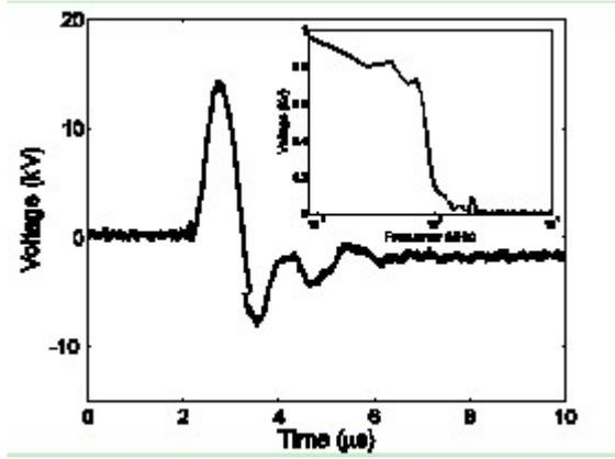
Fig. 2: Measured nanosecond pulse waveform generated across the load and (inset) associated frequency spectral components from DC to 10 MHz.
