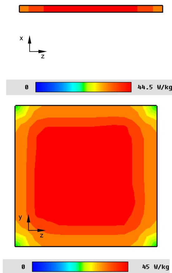
Fig. 4: Energy dose distributions on the  $xz$  plane (left) and  $yz$  plane (right) by simulated specific absorption rate subjected to pulsed electric fields on the liquid sample in the treatment chamber.
