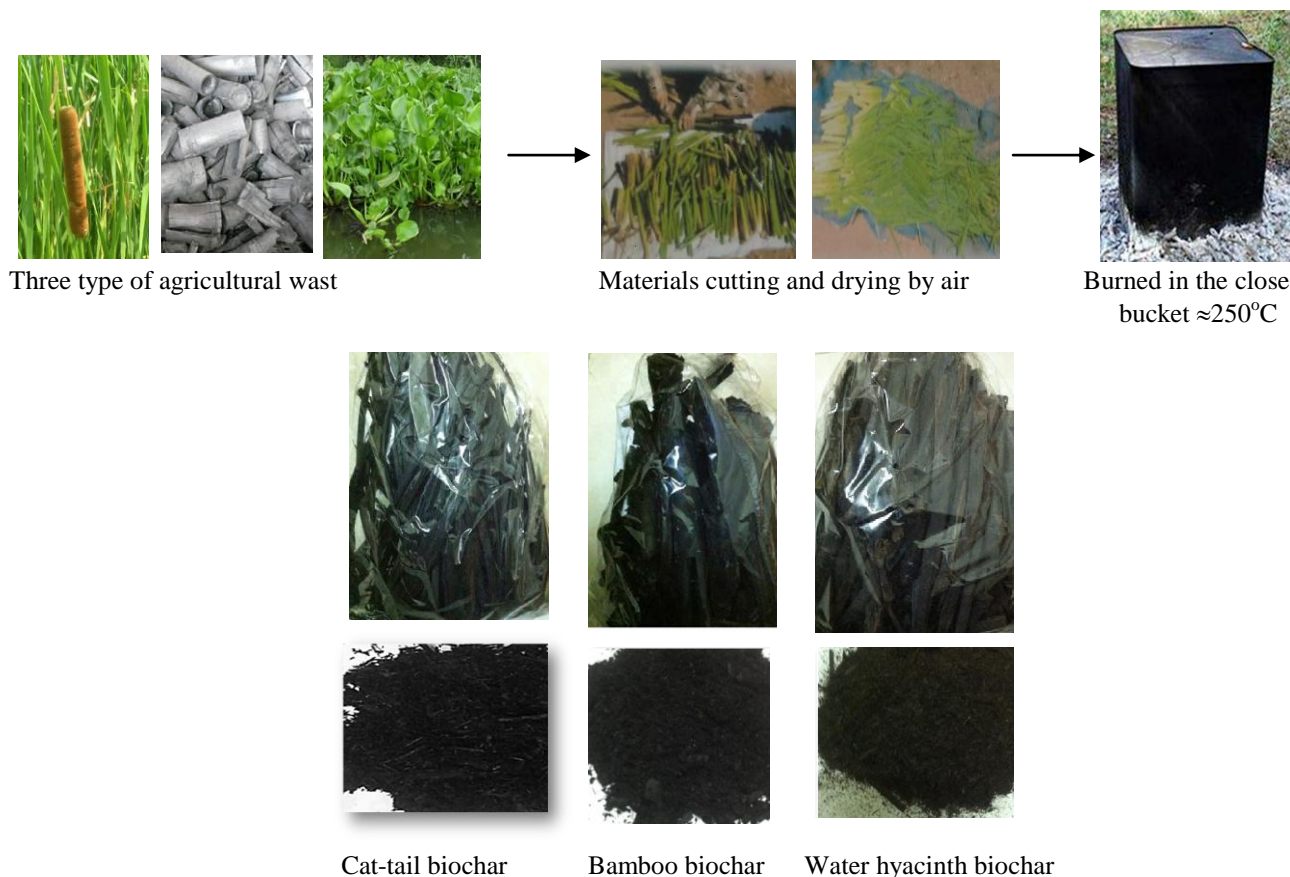
Fig. 1: Preparation of biochar from agricultural residues
