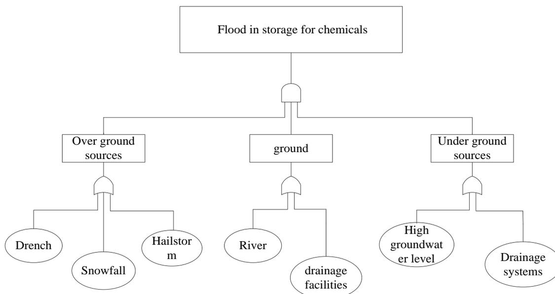
Fig. 1: An example for an application of "Fault tree analysis" method for environmental risk assessment from flood in chemicals substances storages
