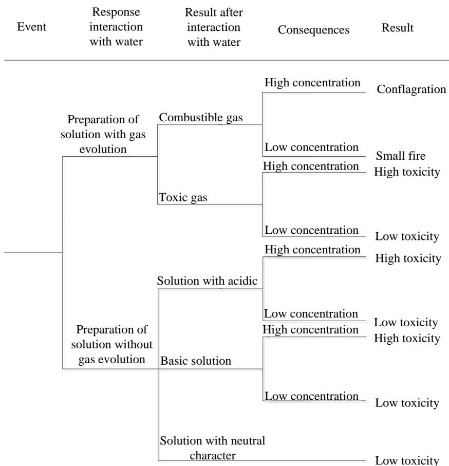
Fig. 2: An exemple for an application of " Tree of events" method for environmental risk assessment from flood in chemicals substances storages
