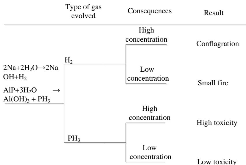
Fig. 3: A diagram of “Tree of events” with specific chemicals
