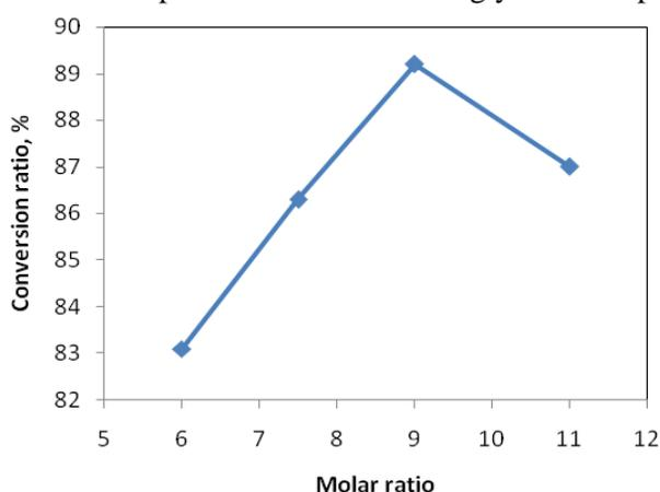
Fig. 2: Effect of molar ratio on conversion ratio.
