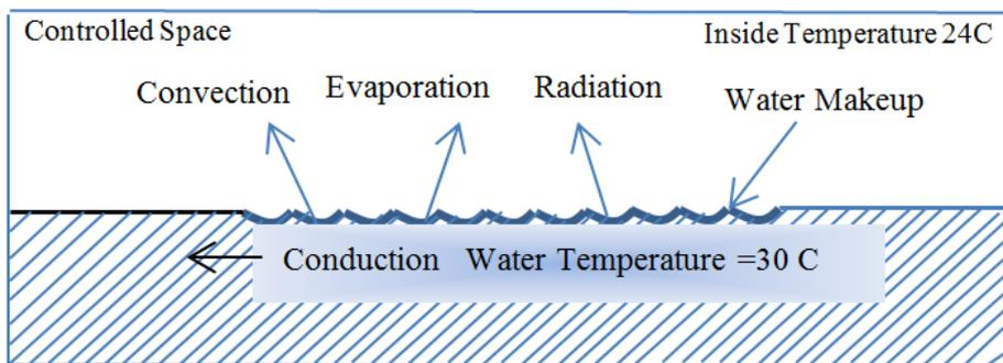
Fig. 2: Schematic diagram of the heat loss
