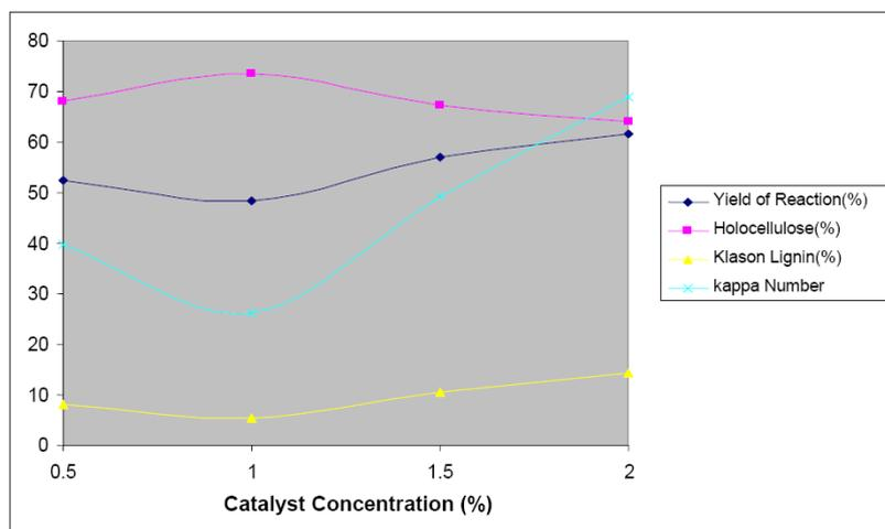
Fig. 2: Effect of catalyst concentration on pulp Yield, holocellulose, klason lignin and Kappa Number
