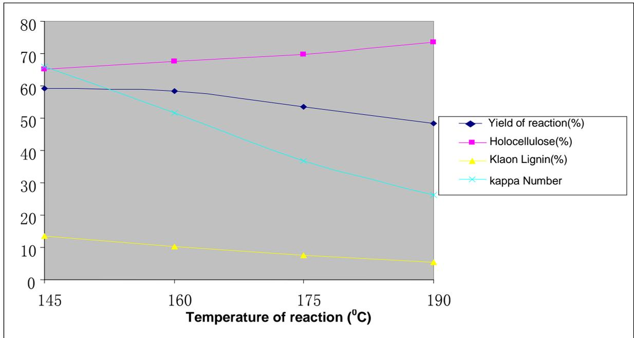
Fig. 4: Effect of temperature of reaction on yield, holocellulose, klason lignin and kappa number
