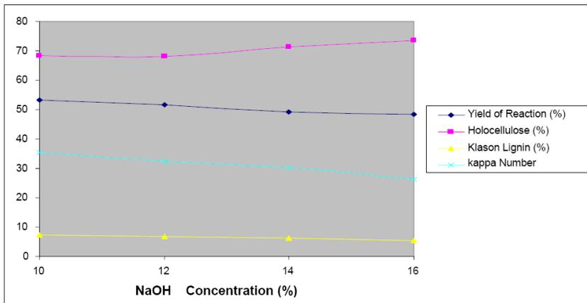
Fig. 1: Effect of Caustic soda concentration on pulp Yield, holocellulose, klason lignin and Kappa Number
