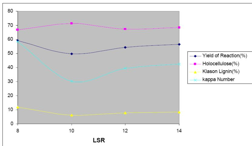
Fig. 3: Effect of LSR (Liquor to Straw Ratio) on pulp Yield, holocellulose, klason lignin and Kappa Number.
