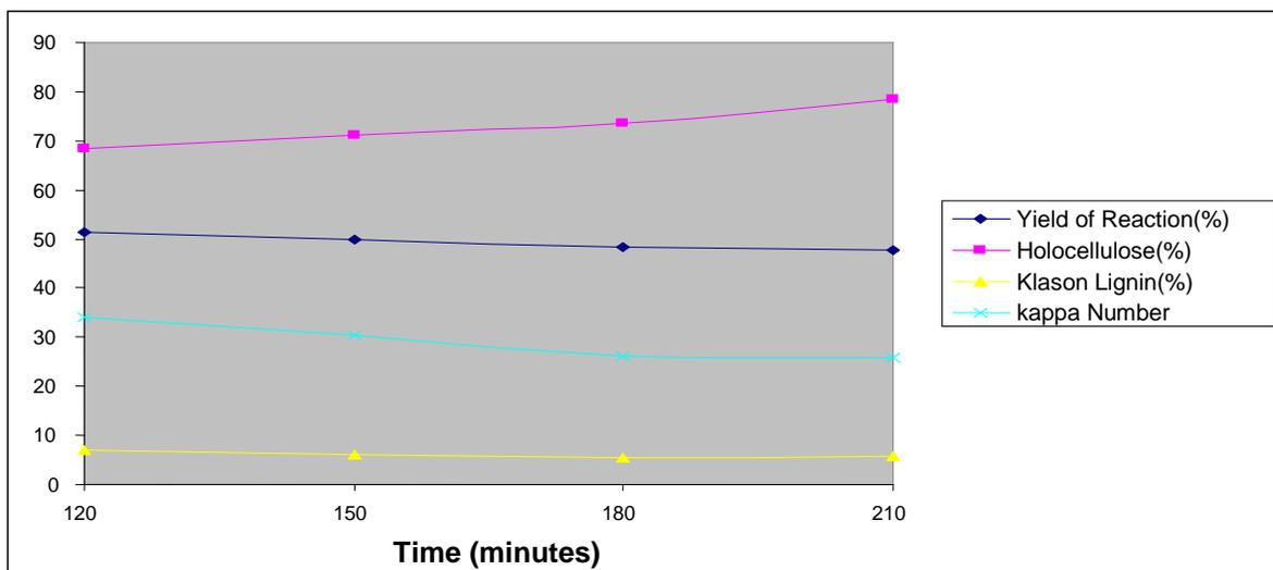
Fig. 5: Effect of time of reaction on yield, holocellulose, klason lignin and kappa number
