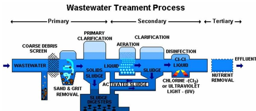
Fig. 1: Typical process of wastewater treatment plants [3]
