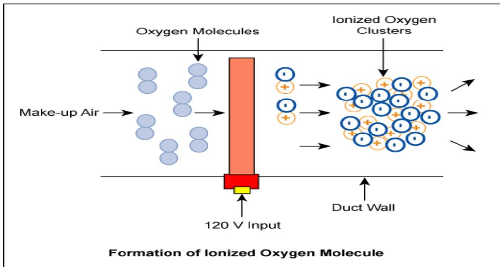
Fig. 2: Illustrations of ionized oxygen clusters [12]
