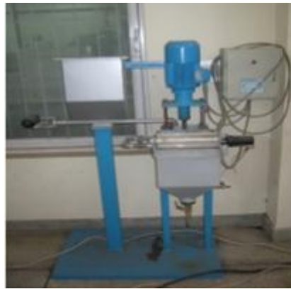
Fig. 1: Rig used for froth flotation
