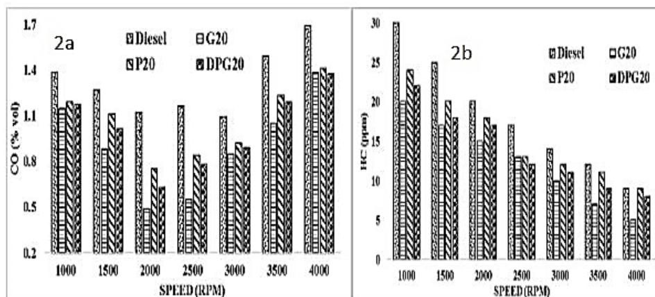
Fig. 2: Variation of CO (2a) and HC (2b) emission of all test fuels.
