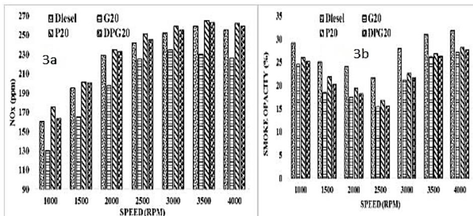
Fig. 3: Variation of NO<sub>x</sub> (3a) and smoke (3b) emission of all test fuels.
