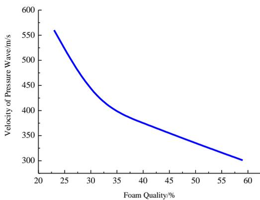
Fig. 4: Changes of the Pressure Wave Velocity in Foam Fracturing Fluid as Foam Quality changes
