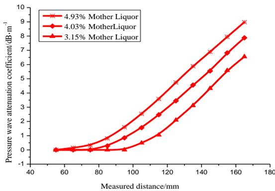
Fig. 7: The Changing Law of Pressure Wave Attenuation Coefficient in Clean Fracturing Fluids With Various Concentrations.
