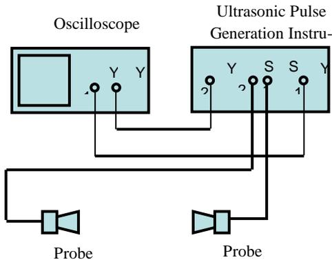
Fig. 1: The diagram of experimental apparatus of measuring pressure wave velocity using pulse method
