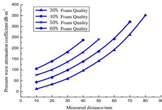
Fig. 9: Changes of Pressure Wave Attenuation Coefficient Variation in Foam Fracturing Fluids with Different Foam Weights.
