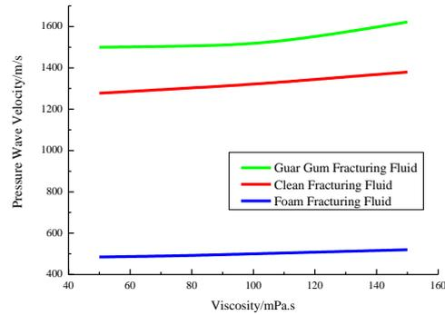
Fig. 2: Changes of the Pressure Wave Velocity in Different Types of Fracturing Fluid as Viscosity Changes
