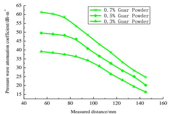
Fig. 7: The Changing Law of Pressure Wave Attenuation Coefficient in Guar Fracturing Fluids With Various Concentrations
