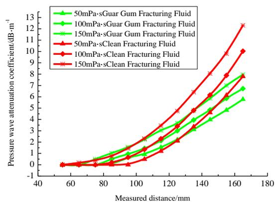
Fig. 5: Changes of Attenuation Index of Guar Gum Fracturing Fluid Pressure Wave and Clean Fracturing Fluid Pressure Wave as the Viscosity changes.
