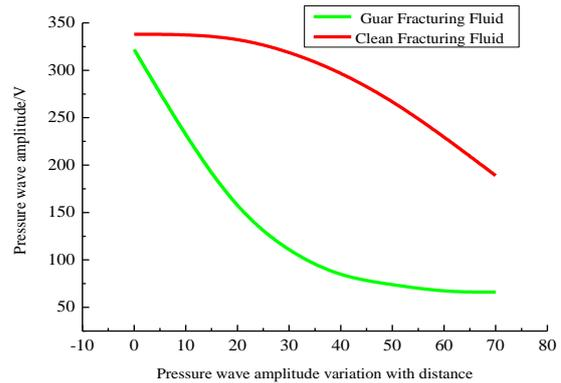
Fig. 8: Changes of Pressure Wave-Amplitudes in Fracturing Fluids as Distances Change.
