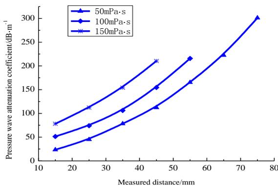
Fig. 6: Changes of Attenuation Index of Foam Fracturing Fluid Pressure Wave as the Viscosity Changes
