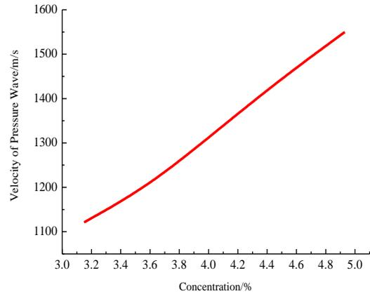
Fig. 3: The Changing Law of the Velocity of Pressure Wave in Clean Fracturing Fluid with Concentration
