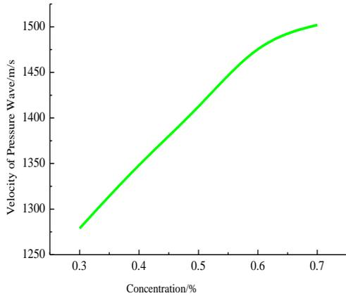
Fig. 3: The Changing Law of the Velocity of Pressure Wave in Guar Gum Fracturing Fluid with Concentration
