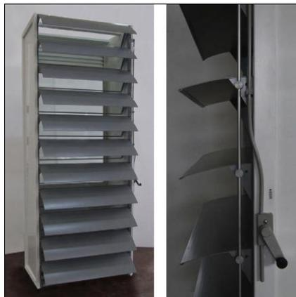
Fig. 1: Prototype of the double skin façade proposed in an open configuration
