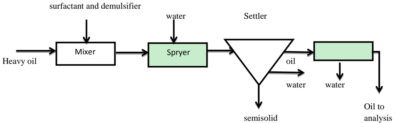
Fig. 5: Process block diagram
