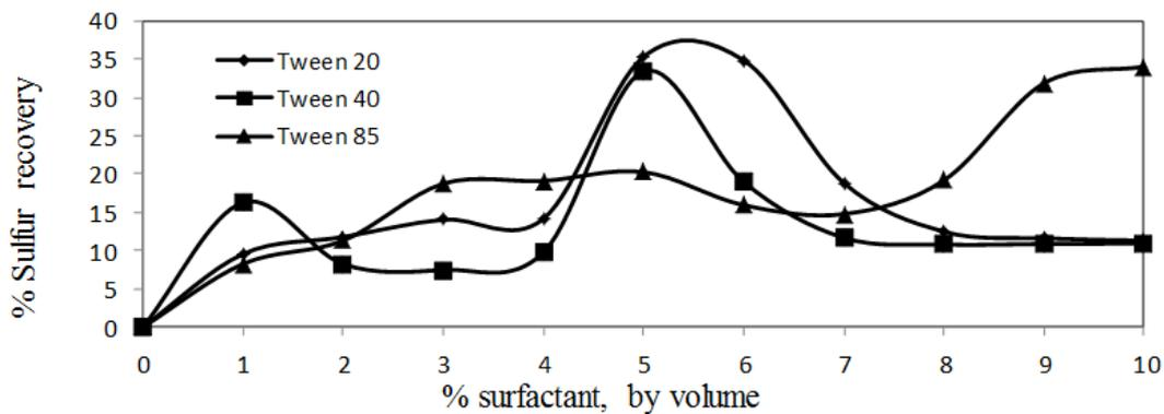
Fig. 6: Sulfur recovery with amount of surfactant
