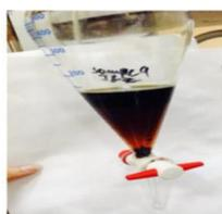
Fig. 4: Three phases of heavy oil, water, and solid deposit formed
