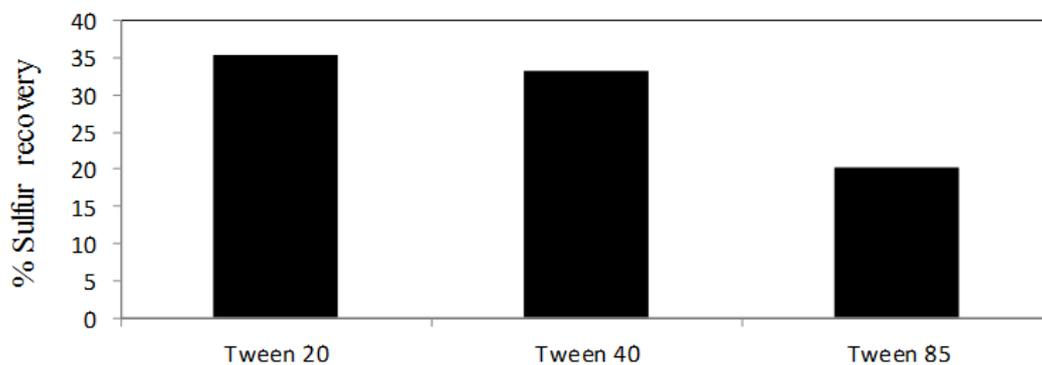
Fig. 7: Sulfur recovery using 5% surfactant
