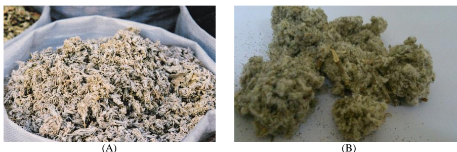
Fig. 1: A) Youda and (B) Masoofa sorbents for oil spill
