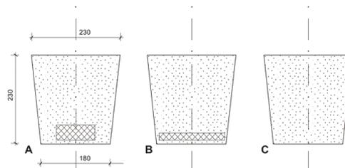
Fig. 1: Outline of the experiment: (a) point geocomposite, (b) geocomposite mat, (c) soil with water
