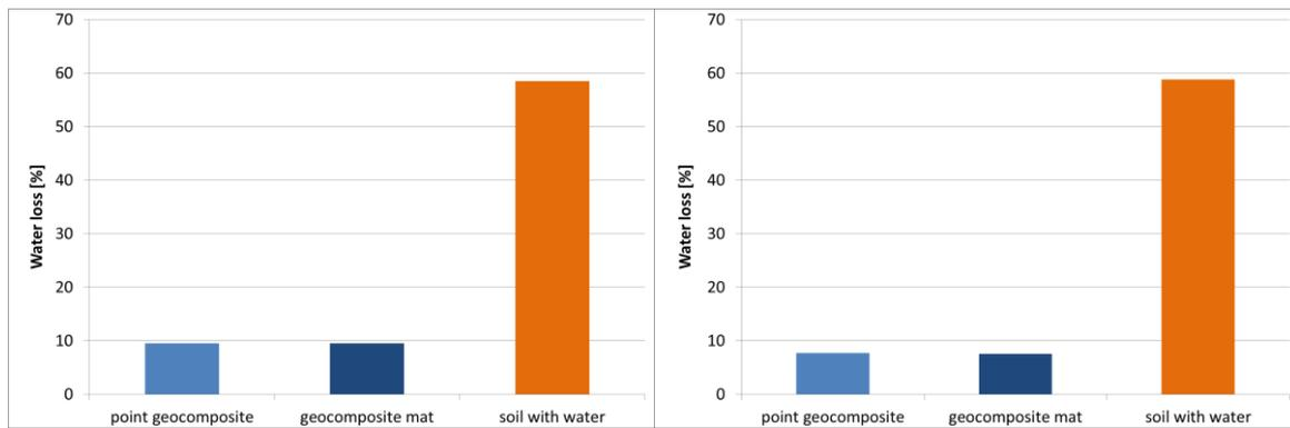
Fig. 3: Water loss percentage with and without geocomposite (a) sandy soil, (b) loamy soil
