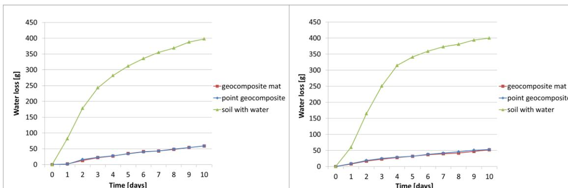
Fig. 2: Water loss with and without geocomposites (a) from sandy soil, (b) from loamy soil
