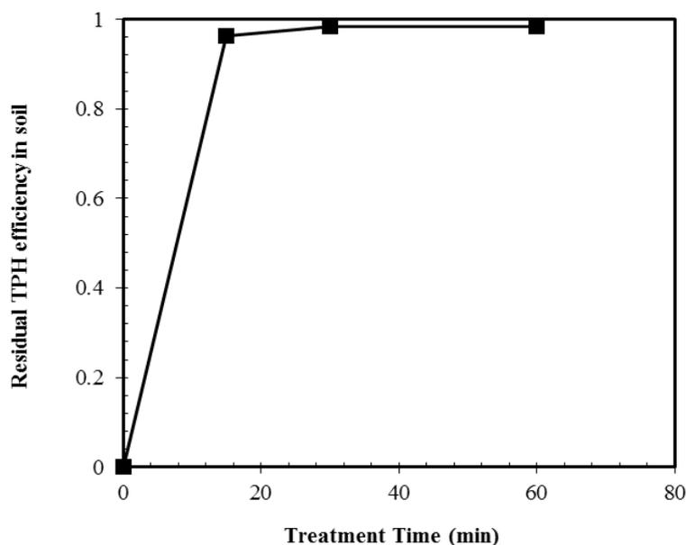
Fig. 6: Removal efficiency of the tested soil treated by microwave thermal desorption
