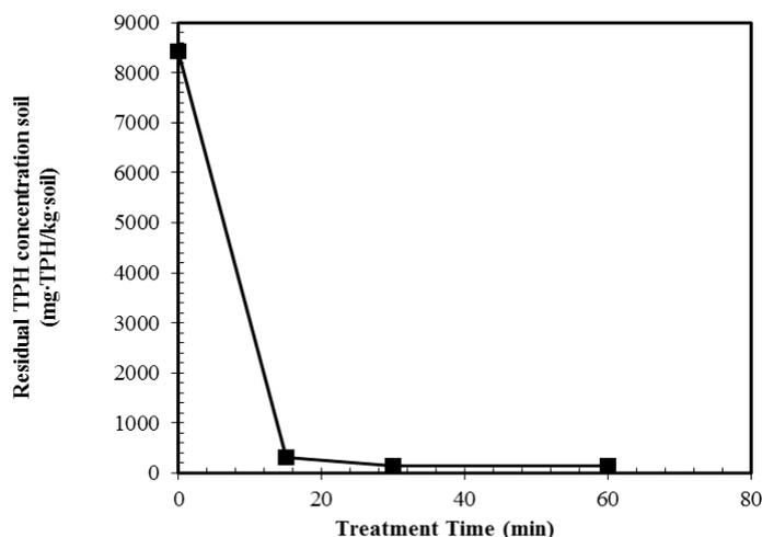
Fig. 5: TPH of the tested soil treated by microwave thermal desorption
