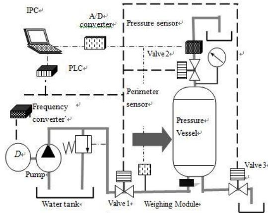
Fig.1: Structure of automatic control system
