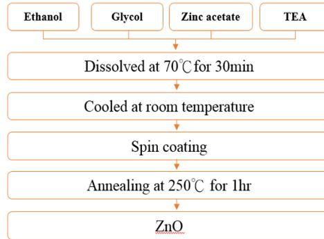
Fig. 1: The preparation process of ZnO thin film
