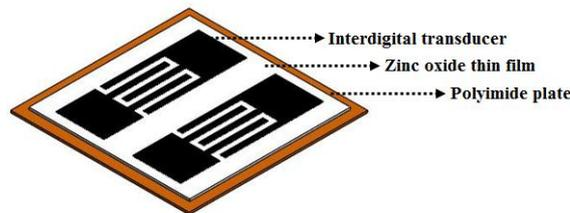
Fig. 2: The flexible carbon dioxide sensor
