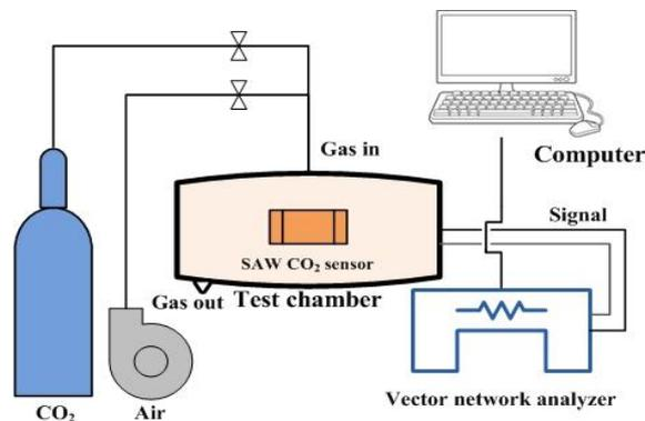
Fig. 3: Schematic diagram of CO<sub>2</sub> sensor measured system
