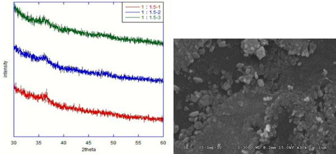
Fig. 4: (a) X-ray diffractogram of the ZnO thin film and (b) SEM image of the ZnO thin film
