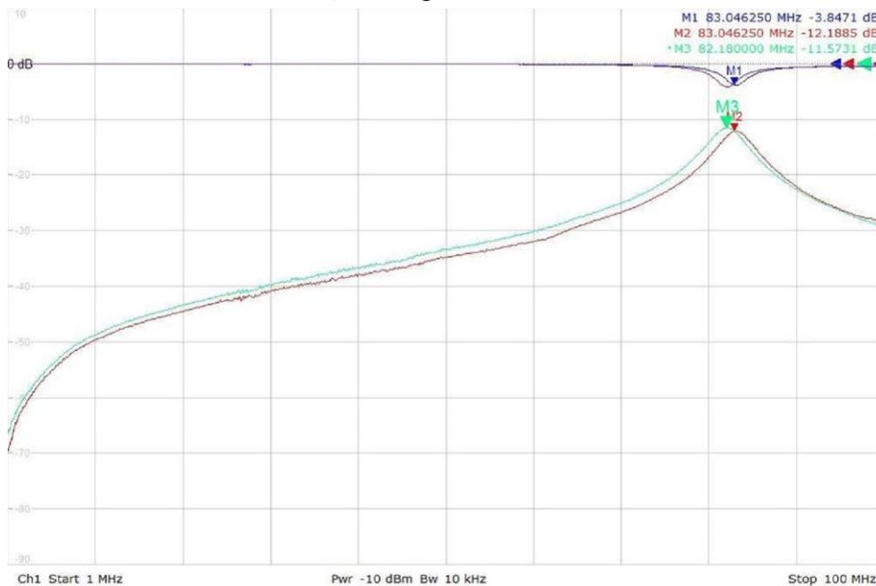
Fig. 5: Sensor response of ZnO thin film to CO<sub>2</sub> by vector analyzer network
