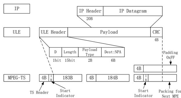
Fig. 2: ULE Encapsulation Principle
