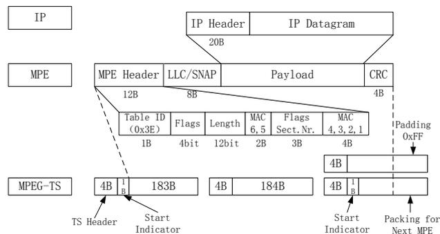
Fig. 1: MPE Encapsulation Principle
