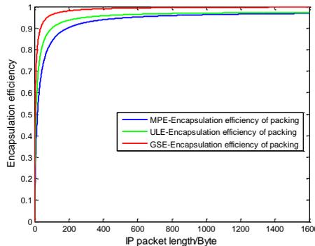
Fig. 5: Encapsulation Efficiency of MPE, ULE and GSE
