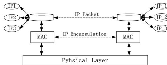
Fig. 6: IP over Satellite Routing and Addressing Mechanism
