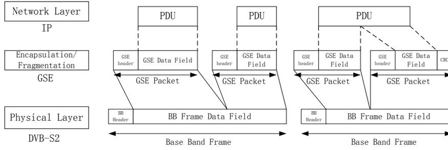
Fig. 3: GSE Encapsulation Principle
