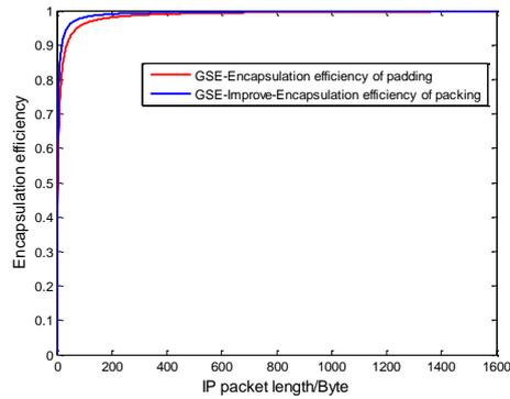
Fig. 11: Efficiency comparison of GSE and GSE-Improve Encapsulation
