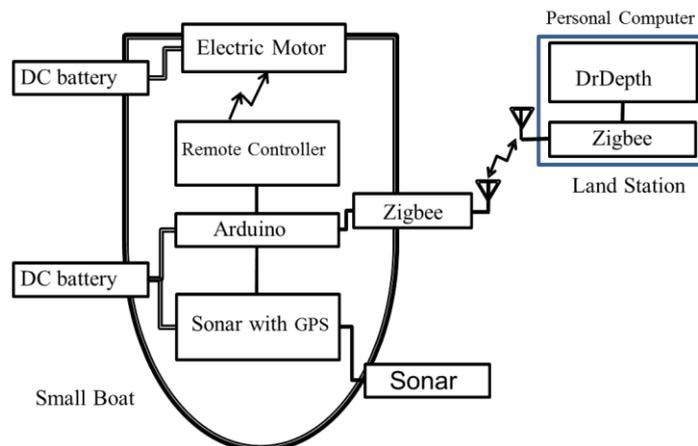
Fig. 1: Schematic diagram of the depth-survey robot
