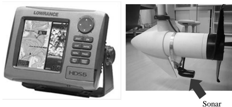
Fig. 2: Sonar with GPS and its attachment
