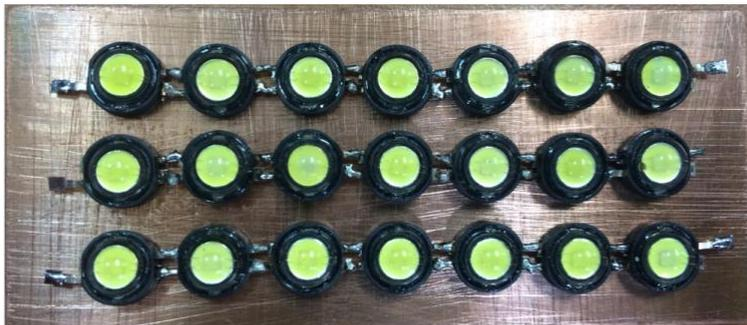
Fig. 1. The high power LEDs array without cooling module.
