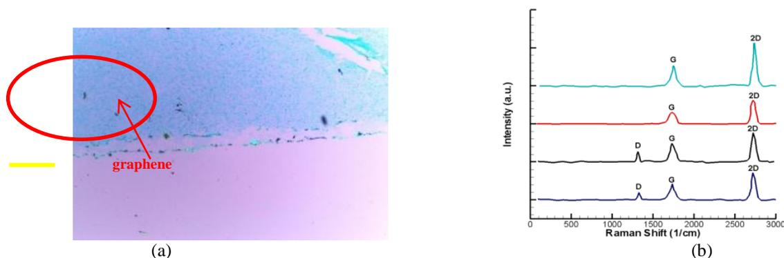
Fig. 2: (a) Optical microscope image shows a CVD-graphene film grown on the Cu-foil after transfer to a Si wafer with 300 nm  $\text{SiO}_2$  layer. (b) Raman spectrum of graphene film grown on  $A_{\text{SUB}}$ ,  $B_{\text{SUB}}$ ,  $C_{\text{SUB}}$  AND  $D_{\text{SUB}}$  substrate; with colored in cyan, red, black and blue, respectively. scale bar: 1  $\mu\text{m}$ .
