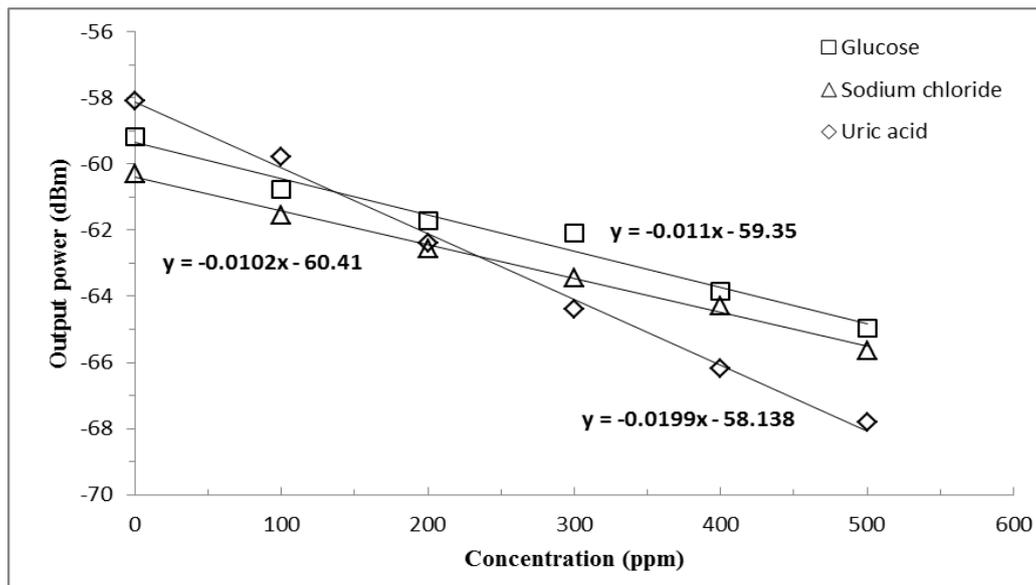
Fig. 4: Output power against the different biochemical concentration.
