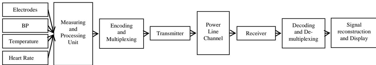
Fig. 2. Block representation of the Health Monitoring System
