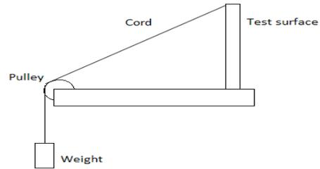
Figure 3. The setup of the test surface and weight to the sample
