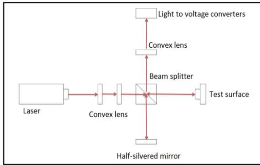
Figure 1. Schematic diagram for the setup of the ESPI system.
