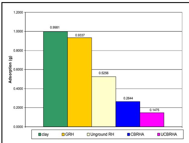
Figure 4. Results of water adsorption for clay, GRH, unground RH, CBRHA and UCBRHA
