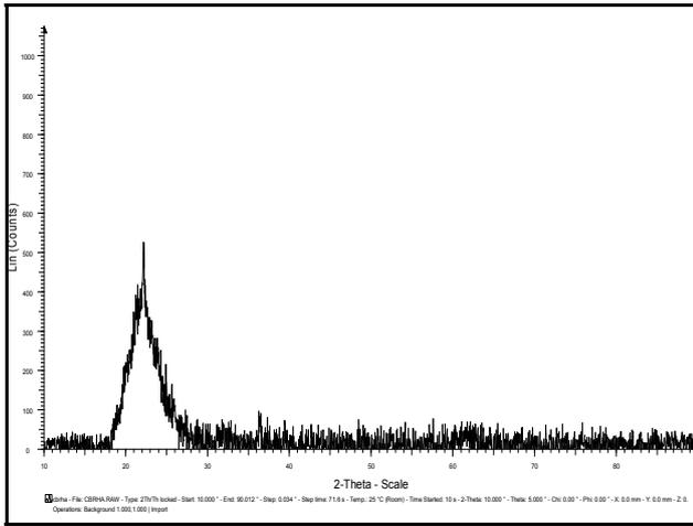
Figure 1. XRD of Controlled Burning Rice Husk Ash (CBRHA)
