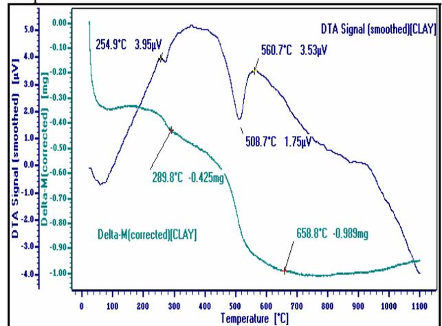
Figure 3. Thermogravimetric analysis of clay
