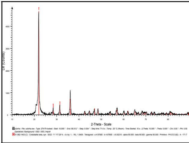
Figure 2. XRD of Uncontrolled Burning Rice Husk Ash (UCBRHA)
