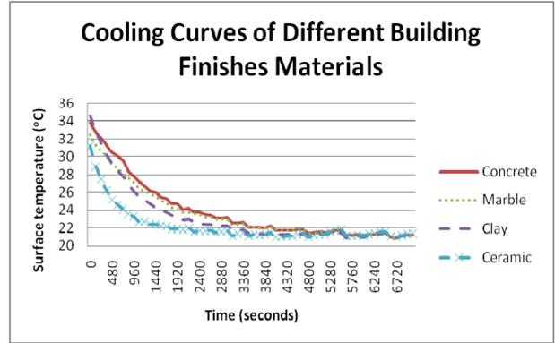
Figure 2. Cooling curves of different building finishes materials
