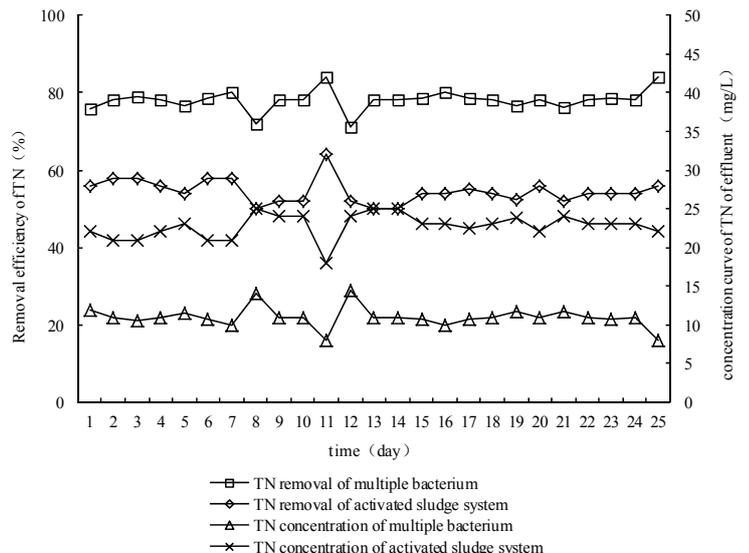
Figure 4. TN effluent concentration and removal rate
