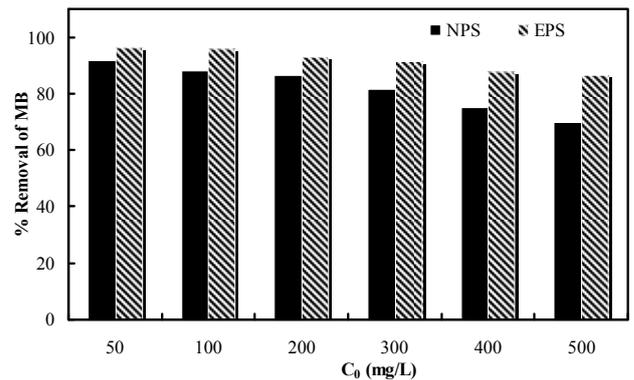
Fig. 1. Influence of chemical modification on adsorption of MB by papaya seed
