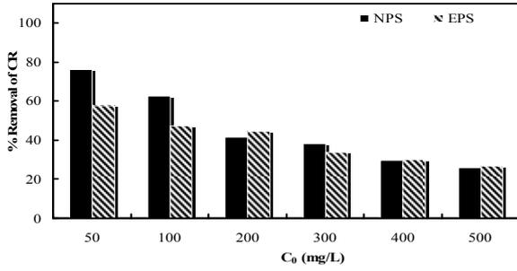
Fig. 2. Influence of chemical modification on adsorption of CR by papaya seed
