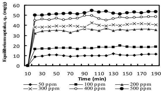
Fig. 4. Effect of contact time and initial concentration on the adsorption of CR on EPS
