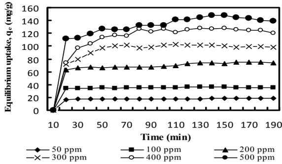
Fig. 3. Effect of contact time and initial concentration on the adsorption of MB on EPS
