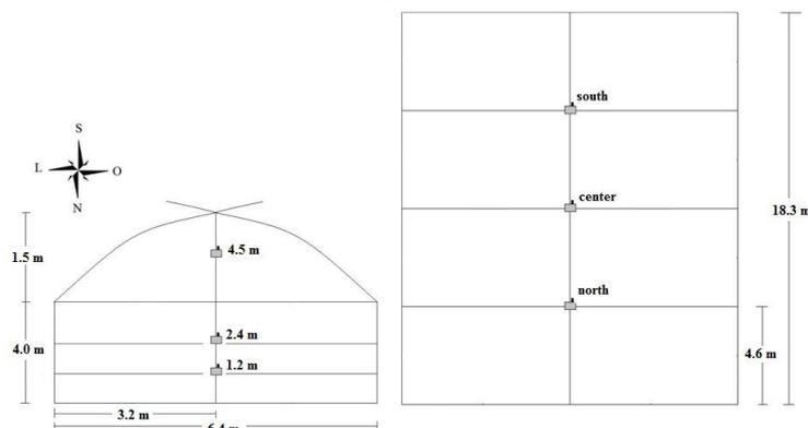
Fig. 2: Wireless sensor network and horizontal and vertical positions of the sensors.
