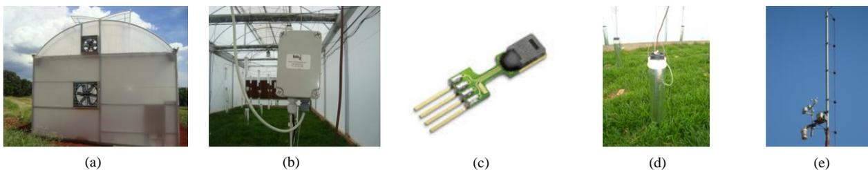
Fig. 1: Greenhouse showing the natural and mechanical ventilation systems (a), with detail to the wireless sensor network (b) and the SHT75 transducer (c) installed inside of PVC tubes (d) and the meteorological station (e).
