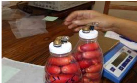
Fig. 1: Enclosure used in respiration measurement setup
